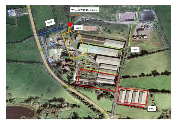
Figure 7-10: Strorm Water Drainage Onsite
